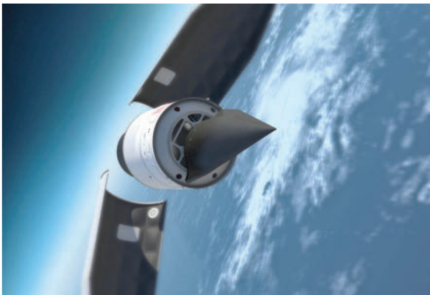
The DARPA Falcon Hypersonic Test Vehicle emerges from its rocket nose cone and prepares to re-enter the Earth’s atmosphere.
