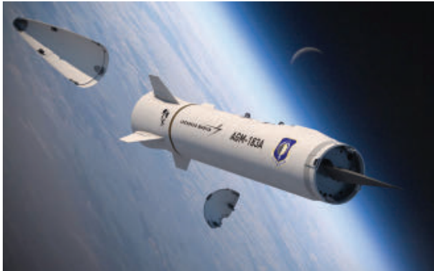
The Lockheed Martin AGM-183 Air-Launched Rapid Response Weapon (ARRW) is an experimental U.S. Air Force hypersonic weapon that uses a boost glide vehicle propelled to a maximum speed of Mach 20.
